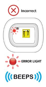
If you see the status light is **FLASHING RED**, and your on-body injector is beeping, your on-body injector is not functioning properly.
